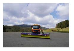
When fully unfolded, the snow plough has an outstanding working width of 6.2 m. When the left wing is folded in, the working width reduces to 5.1 m, and when the right wing is folded in, it reduces to 4.5 m. When both wings are fully folded, the clearing width is 3.4 m, while the wings can folded hydraulically in both transport and clearing positions, minimising the transport width. They are automatically raised during the clearing operation.
