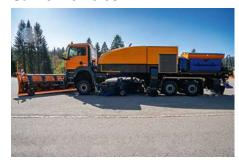
As standard, the CJS-DI seamlessly mounts onto the MAN TGS 18.320 chassis type carrier vehicle. This carrier vehicle features a turning circle diameter of 18 meters and offers the option for additional rear axle steering for enhanced agility. The basic equipment and the exhaust emissions of the carrier vehicle must be selected specifically to meet the standards of the customer and the relevant country.
