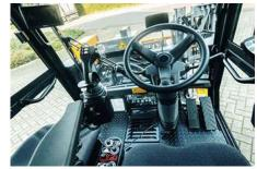
steering column including a tilt function ensures a comfortable position – even for larger drivers. Ergonomically designed operating controls and a fully air-conditioned cabin guarantee a relaxed working environment. The driver controls operations manually using a joystick.
